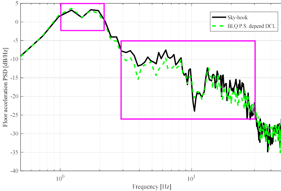
Fig. 2-19 Comparison of floor acceleration PSD on swell and head toss road 73km/h
