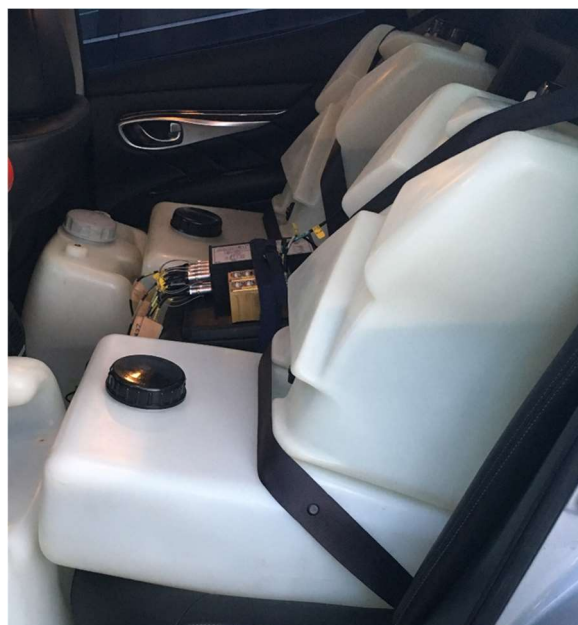
Fig. 4-17 Increasing Rear Sprung Mass Weight
