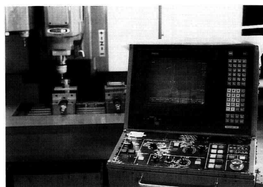
Fig. 2(b) NC controller for machine tool
