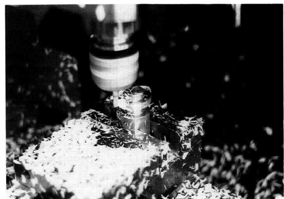
Fig. 8(b) Cutting of plate cam (finishing)
