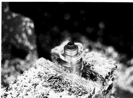
Fig. 9. Finished plate cam
