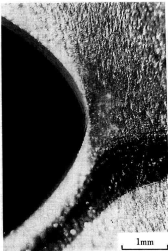
Fig. 4-5. Profile of the opened tip of the crack.
