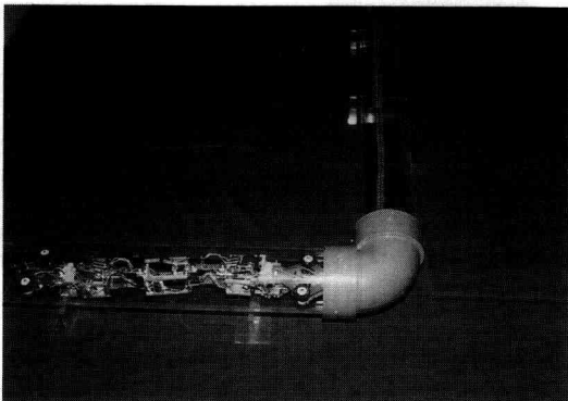
Photo 4-5. Locomotion through elbow pipe (4)
