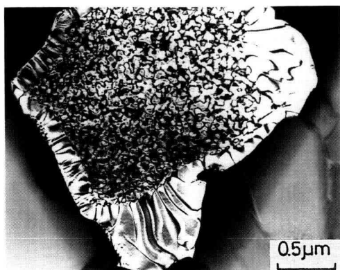
Fig. 1-1. Dark field electron micrograph of APDs formed during melt quenching in \text{Ni}_3\text{Al} alloy, showing that swirl-like APDs are formed inside the grain and stripe-like APDs are formed near the grain boundary.
