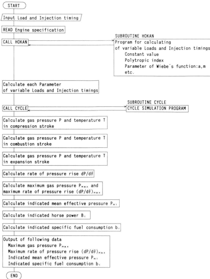
Fig. 4. Flow chart of combustion cycle simulation.
